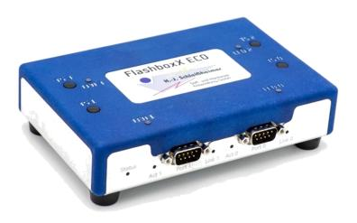
The FlashboxX ECO is a hardware device designed to flash Automotive ECUs via several BUS systems. It features a Linux-based software environment, pre-installed for tasks such as flashing ECUs according to the VW Standard, data set comparison, and functioning as a gateway or datalogger. The software is fully customizable to meet customer-specific requirements, it can be adapted either by the user or by the manufacturer.
