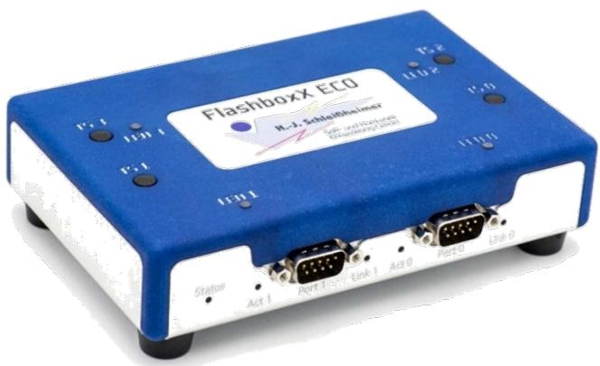
The FlashboxX ECO is a hardware device designed to flash Automotive ECUs via several BUS systems. It features a Linux-based software environment, pre-installed for tasks such as flashing ECUs according to the VW Standard, data set comparison, and functioning as a gateway or datalogger. The software is fully customizable to meet customer-specific requirements, it can be adapted either by the user or by the manufacturer.
